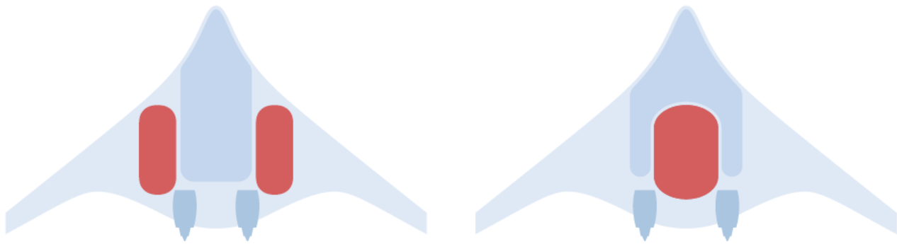
Figure 121 - Two potential arrangements for hydrogen tanks in a BWB configuration. The darker area shows the passenger cabin [01]
