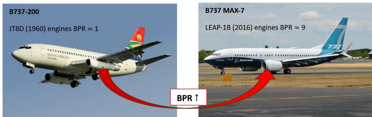
Figure 5 - Comparison of BPR between 737-200 and 737MAX-7 engines
