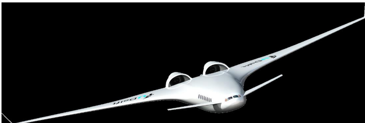
Figure 52 - Blended Wing Body (BWB) concept developed for the AHEAD project [17]
