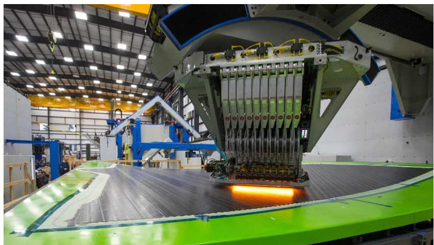
Figure 1 - Electroimpact machines lay down thin strips of carbon fiber infused with epoxy resin (Source: The Ledger)
