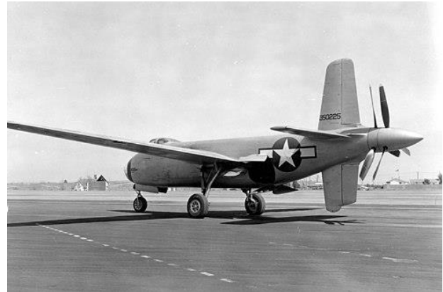
Figure 15 - View of the contraprop and cruciform tail [23]
