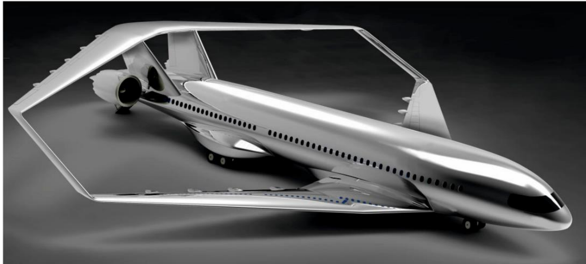
Figure 79 - Representation of the PrandtlPlane (PrP) under development within the project "PrandtlPlane ARchitecture for the Sustainable Improvement of Future AirpLanes" (PARSIFAL) [18]
