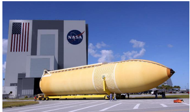
Figure 118 - The LH 2 external tank of the space shuttle covered in a layer of sprayon foam insulation (the orange material) that was 1-2 inches thick [01]
