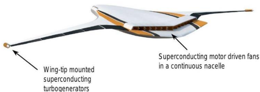
Figure 39 - NASA N3-X Distributed Turboelectric Propulsion System
