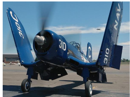
Figure 70 - Corsair F4U-4 folding its wings Source: Wikipedia
