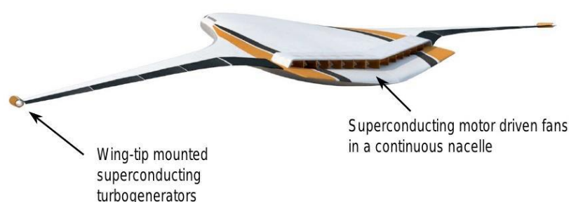
Figure 103 - NASA CONCEPT: N3-X Distributed Turboelectric Propulsion System. (Credit: NASA)
