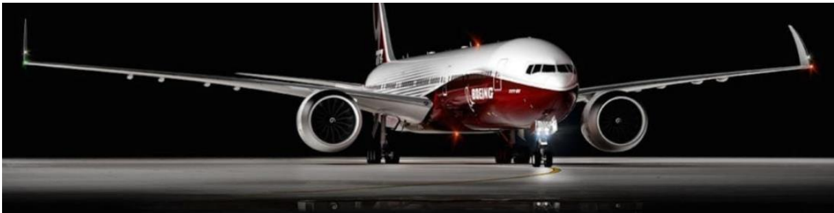
Figure 72 - 777X with its wingtips folded [08]
