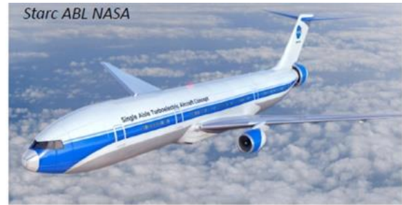
Figure 36 - Single-aisle turboelectric aircraft with an aft boundary layer propulsor STARC ABL
