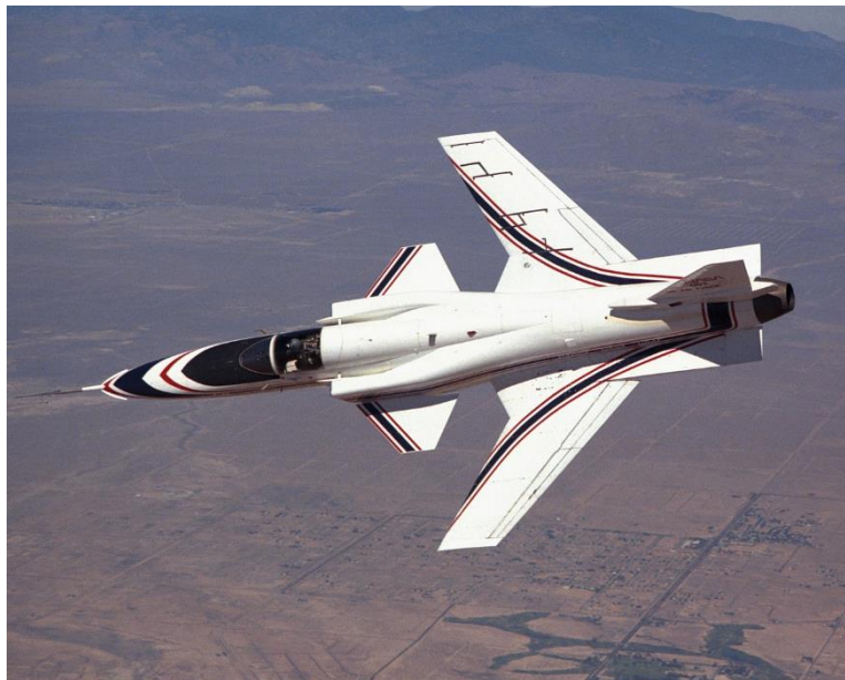
Figure 62 - Grumman X-29 displaying forward-swept wing configuration, Source: NASA Photo Number: EC87-0182-14, Public Domain, https://commons.wikimedia.org/w/index.php?curid=1479146
