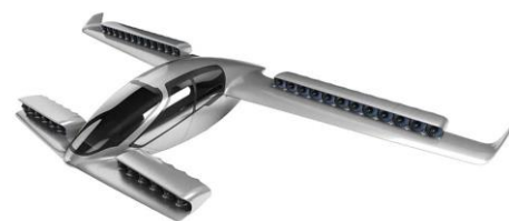
Figure 37 - VTOL Lilium Jet for autonomous air transportation of 5 passengers
