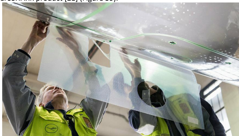
Figure 59 - AeroSHARK film installation [21]
