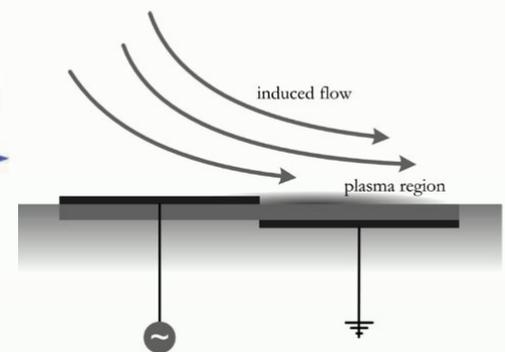
Figure 50 Acceleration of the airflow plasma
