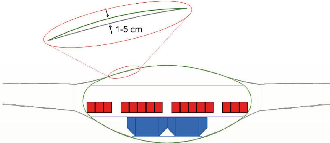
Figure 56 - Cross-section through the oval fuselage showing the cabin and cargo with a detail of the difference between the aerodynamic and pressure shell [25]
