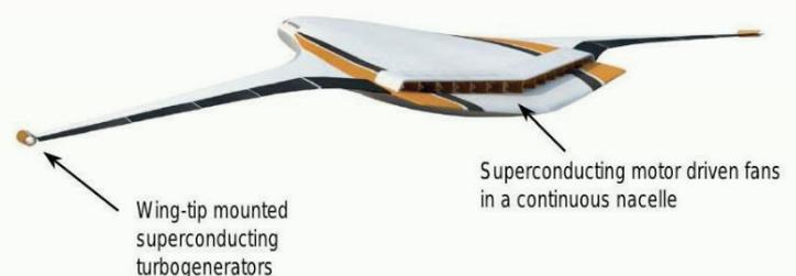
Figure 39 - NASA N3-X Distributed Turboelectric Propulsion System
