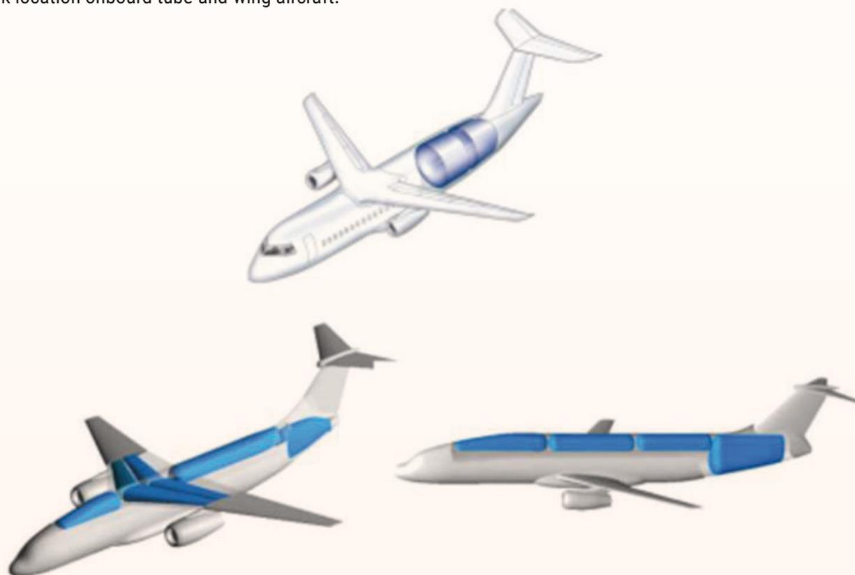
Figure 120 - Liquefied hydrogen aircraft with different tank configurations [10]
