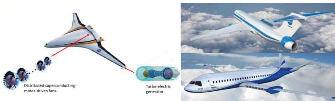
Figure 96 - NASA N3-X and STARC-ABL, and ESAero's ECO-150 (photo: ESAero, San Luis Obispo, California) aircraft concepts [09]
