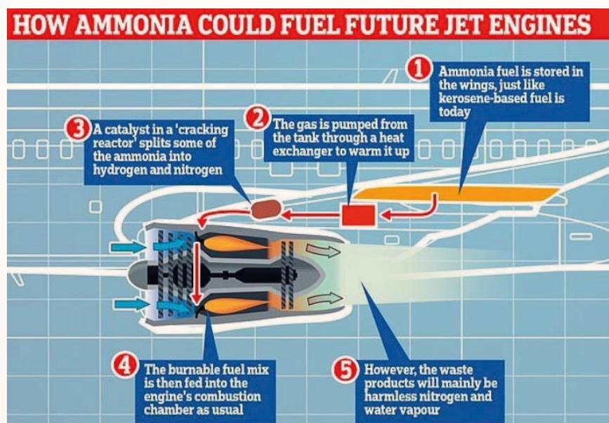
Figure 137 - Simplified view of ammonia combustion jet engine
