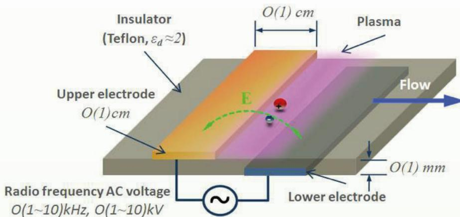
Figure 49 Principle of the plasma actuator
