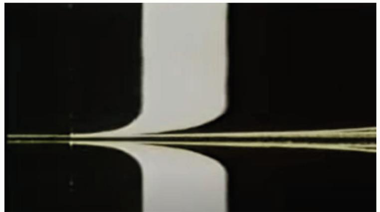
Figure 31 - Boundary layer on a flat plate, water with hydrogen bubbles [2]
