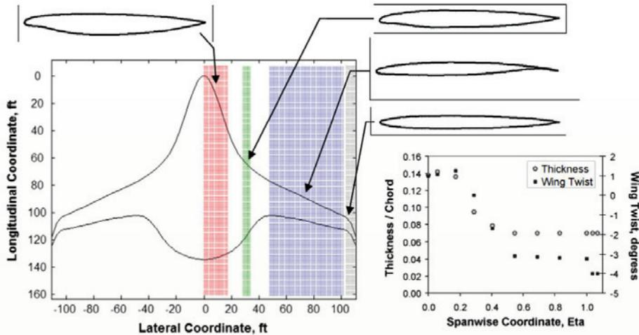
Figure 53 - Example of BWB cross section [24]
