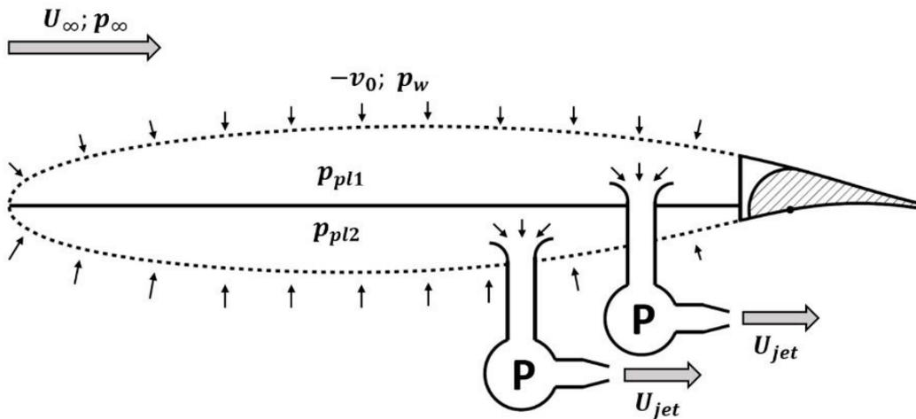
Figure 46 - Components of Suction System: aspiration can be on the whole wing (as above) or just limited to the leading-edge area [08]
