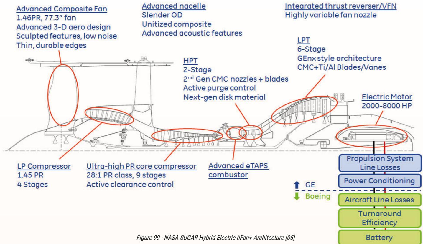
Figure 99 - NASA SUGAR Hybrid Electric hFan+ Architecture [05]
