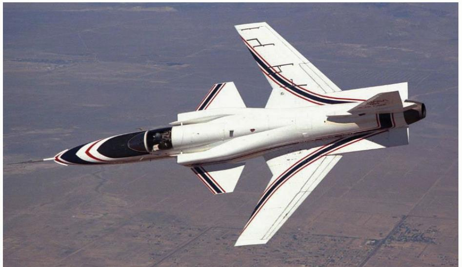
Figure 62 - Grumman X-29 displaying forward-swept wing configuration, Source: NASA
