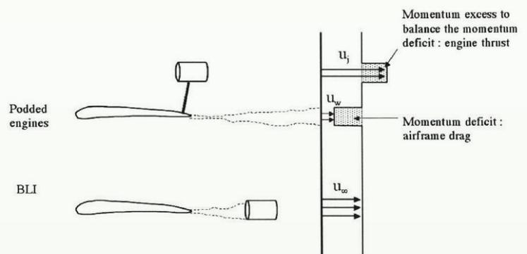
Figure 35 - Illustration of boundary layer ingestion effect on wing downstream flow velocity pattern
