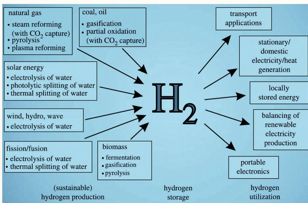
Figure 115 - Hydrogen as an energy carrier linking multiple hydrogen production methods, through storage to various end-users. Highlighted production routes (in red) can involve substantial CO<sub>2</sub> generation [03]
