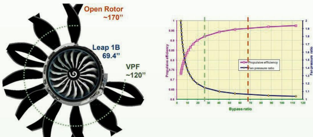
Figure 20 - Propulsive efficiency with By-pass Ratio and Fan pressure Ratio [7]
