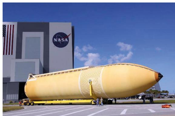
Figure 118 - The LH<sub>2</sub> external tank of the space shuttle covered in a layer of spray-on foam insulation (the orange material) that was 1-2 inches thick [01]
