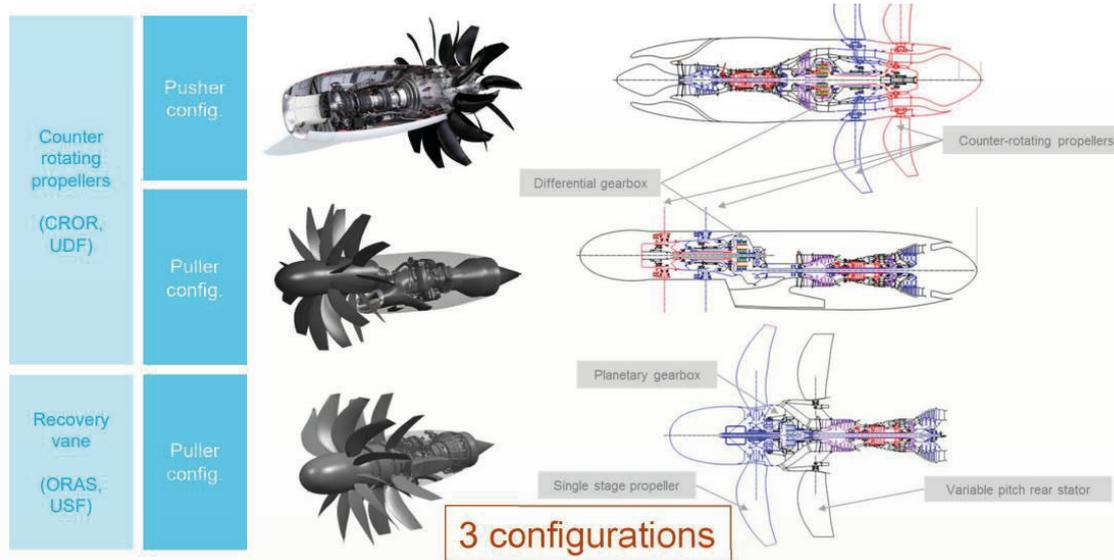
Figure 21 - Different configurations of Open Rotor [7]
