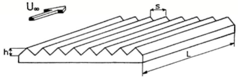
Figure 44 - Riblets surfaces are made of grooves aligned with the flow [11]
