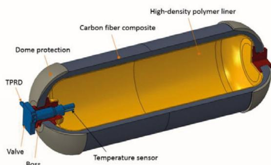
Figure 119 - Tank components for storing hydrogen [14]
