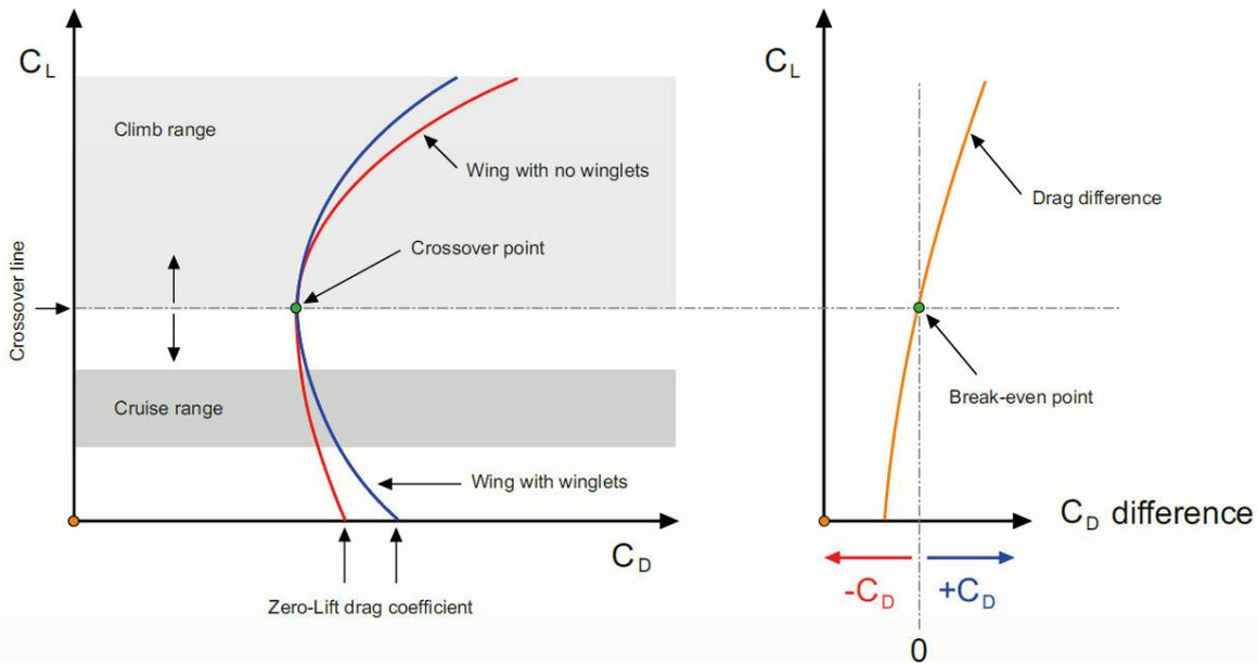
Figure 74 - Comparison of drag polars for a clean wing and a wing with winglet installed ( $C_D$  is the drag coefficient and  $C_L$  is the lift coefficient). On the left image, grey areas represent the climb range and the cruise range of the wing. The right image shows the drag difference, where negative  $C_D$  means drag increment and positive  $C_D$  means drag reduction. The  $C_D$  difference is the  $C_D$  delta between the wing with winglets and the wing without winglets [09]
