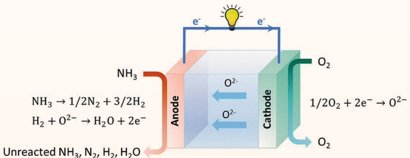
Figure 138 - Simplified view of SOFC-O
