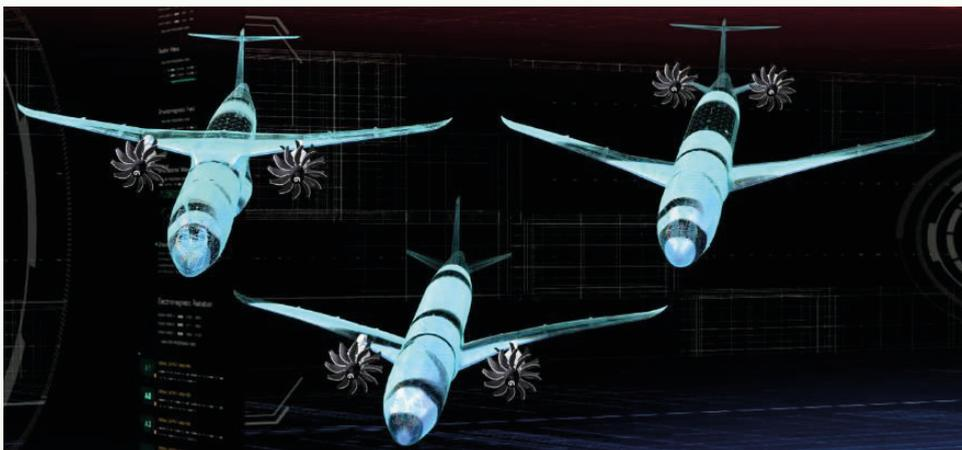
Figure 25 - Open Rotor integration possibilities on classical tube and wing aircraft design [17]
