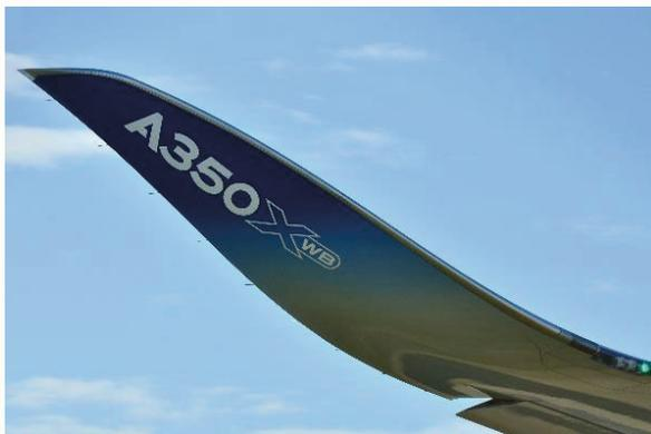
Figure 69 - Blended Winglet of A350XWB
