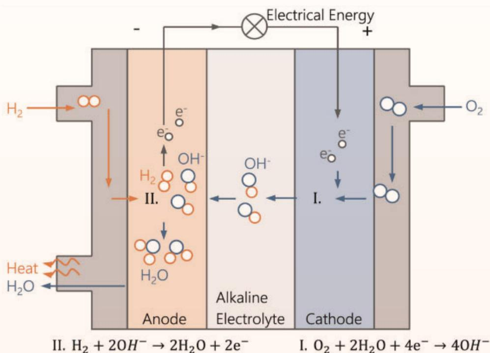
Figure 105 - Alkaline Fuel Cell
