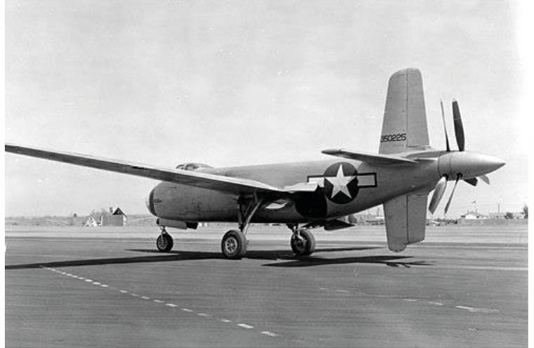
Figure 15 - View of the contraprop and cruciform tail [23]
