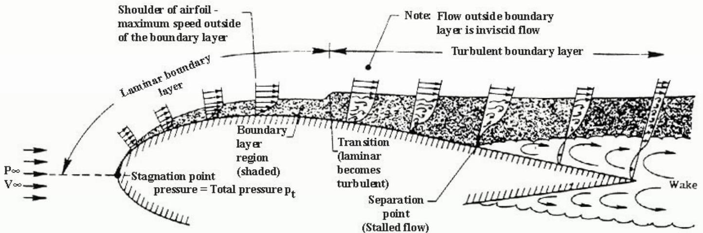
Figure 34 - Flow complexity around a wing section
