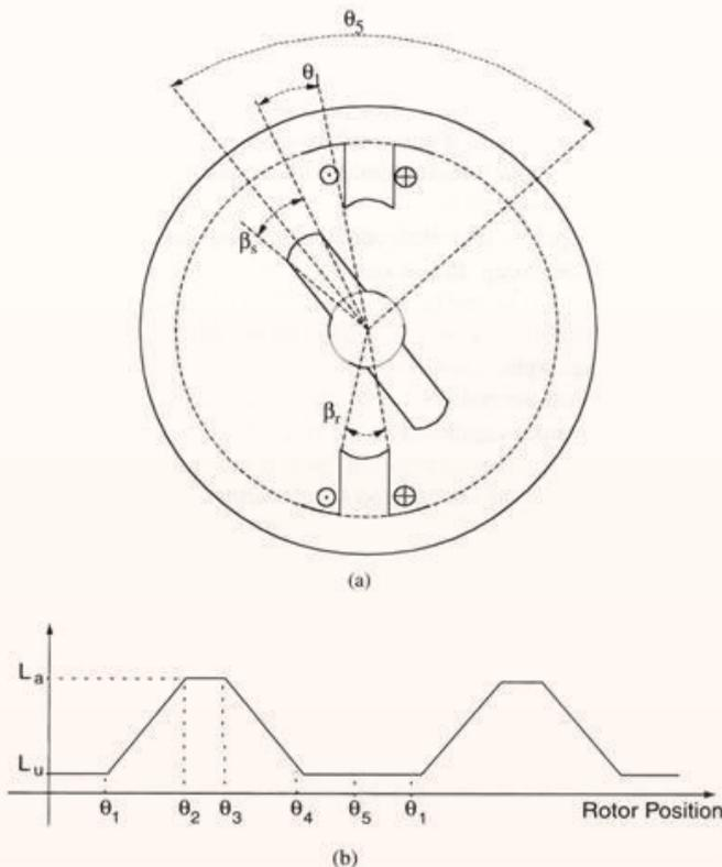
Figure 88 - Example of basic SRM:  $\theta_1 = 12(2\beta_r - (\beta_s + \beta_r))$ ;  $\theta_2 = \theta_1 + \beta_s$ ;  $\theta_3 = \theta_2 + (\beta_r - \beta_s)$ ;  $\theta_4 = \theta_3 + \beta_s$ ;  $\theta_5 = \theta_1 + \theta_4 = 2\beta_r$  [14]
