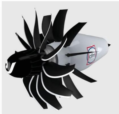
One of their announcements is the design of a commercial Open fan (Figure 24), the most ambitious architecture, for an entry into service by mid of 2030s.
