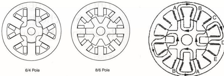
Figure 89 - Examples of industrial SRM engine, with the optimized shape of the rotor close to the magnetic field generated by the stator's windings [14]
