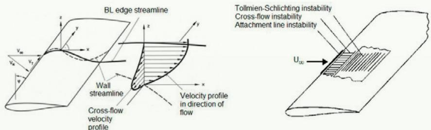
Figure 43 - 3D Boundary Layer on a Swept Wing and related Transition Mechanisms [08]
