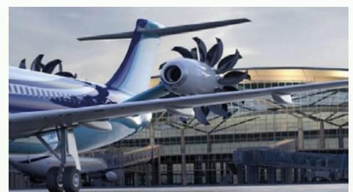
Figure 26 - Open rotor at the back of the aircraft [11]
