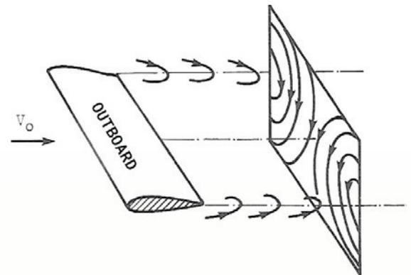
Figure 63 - Generation of the wingtip vortex [01]
