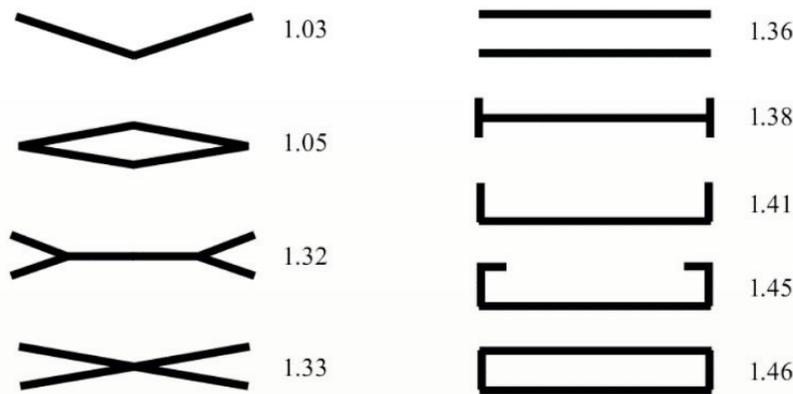
Figure 68 - Indicative values of e, the span efficiency factor for several basic shapes of wing [13]
