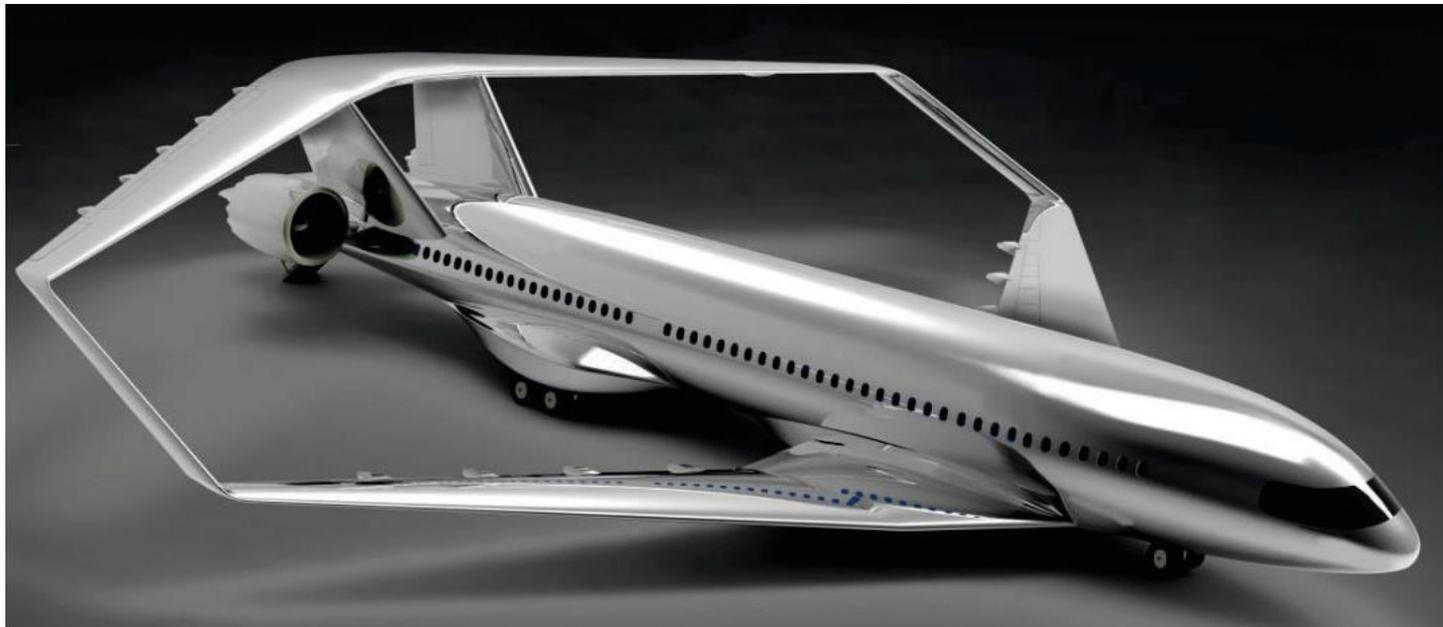
Figure 79 - Representation of the PrandtlPlane (PrP) under development within the project "PrandtlPlane Architecture for the Sustainable Improvement of Future AirLanes" (PARSIFAL) [18]
