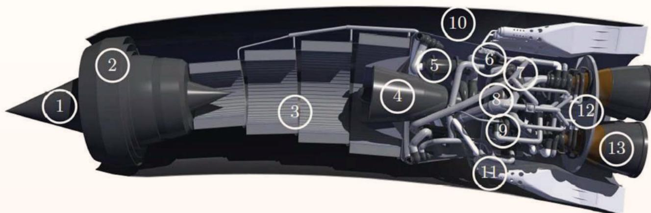
Figure 129 - SABRE section: 1) movable spike 2) intake 3) precooler 4) air compressor 5) preburner and reheater (HX3) 6) helium circulator 7) H<sub>2</sub> pump 8) He turbine and regenerator (HX4) 9) LOx pump 10) spill duct 11) ramjet burn [05]
