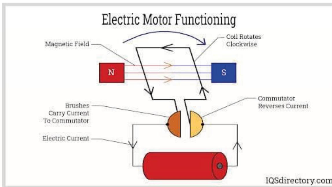
Figure 84 - Basic electric motor with DC supply and brush commutator. Source: IQSdirectory.com
