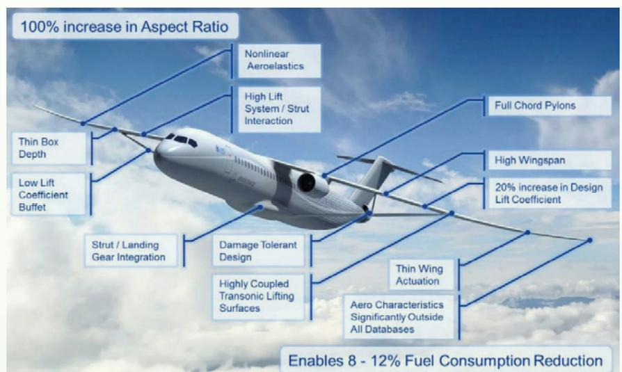
Figure 75 - Transonic Truss-Braced Wing (TTBW) [07]
