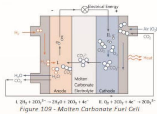
They all have the same one-step reaction using hydrogen as a fuel and oxygen as the oxidizer. They furthermore only reject water (the compounds in gaseous form have the subscript g):  $2H_{2(g)} + O_2(g) \rightarrow 2H_2O_{(g)} + Heat$
