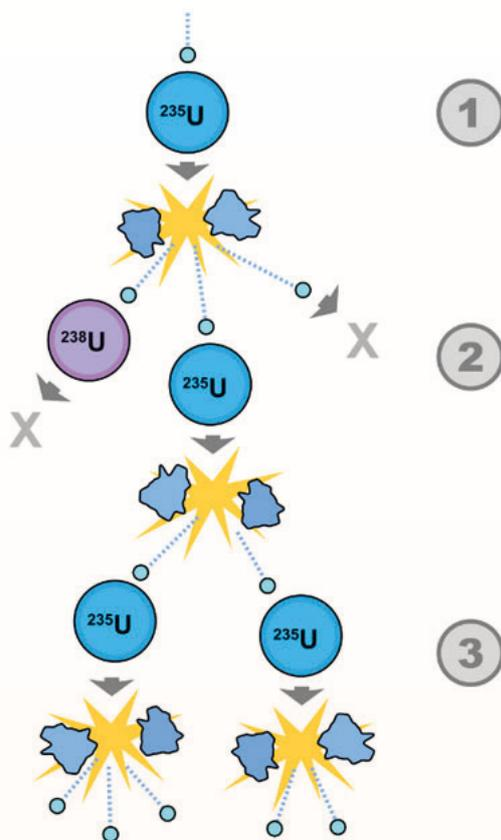
Figure 147 - Schematic diagram of a fission chain reaction. Based roughly on the illustration in the Smyth Report (1945). Caption A uranium-235 atom absorbs a neutron, and fissions into two new atoms (fission fragments), releasing three new neutrons and some binding energy. Both of those neutrons collide with uranium-235 atoms, each of which fission and release between one and three neutrons, and so on. Source: Wikimedia Commons
