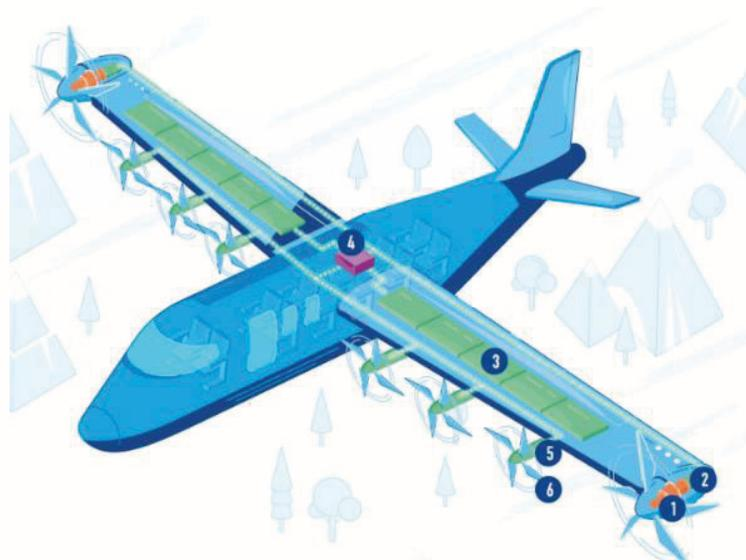
The series hybrid architecture consists of electric motors, with electricity provided from batteries, and kerosene-supplied gas turbines (Figure 101).
