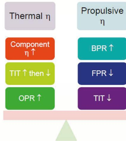
Figure 19 - Levers to increase engines' efficiencies
