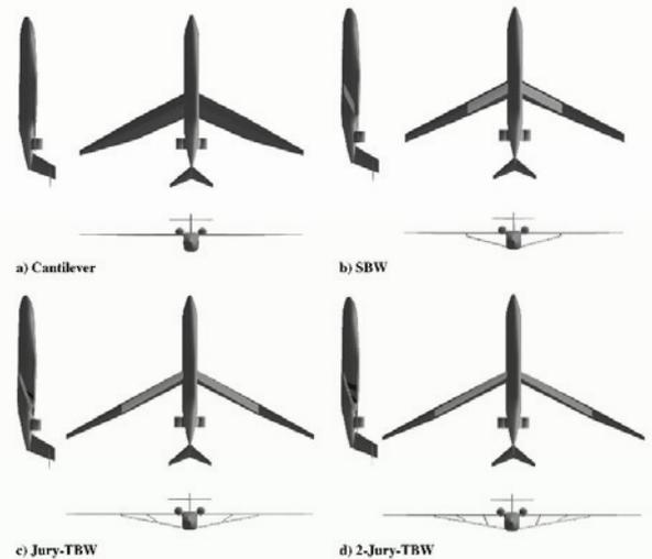
Figure 77 - Baseline optimized minimum-fuel configurations [10]
