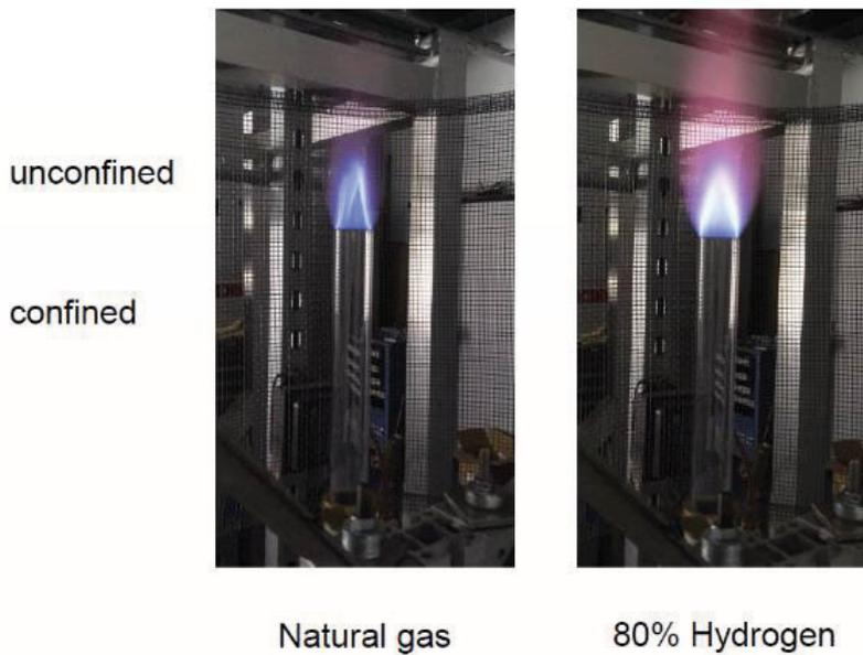
Figure 126 - Comparison of flames between hydrogen and natural gas (hydrocarbon) [07]
