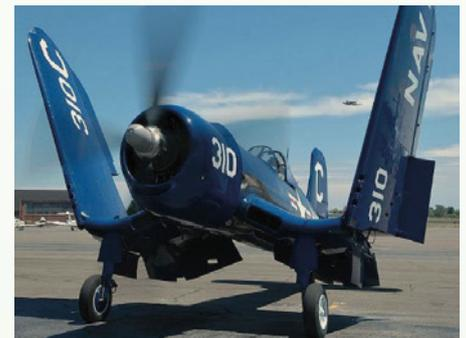
Figure 70 - Corsair F4U-4 folding its wings
