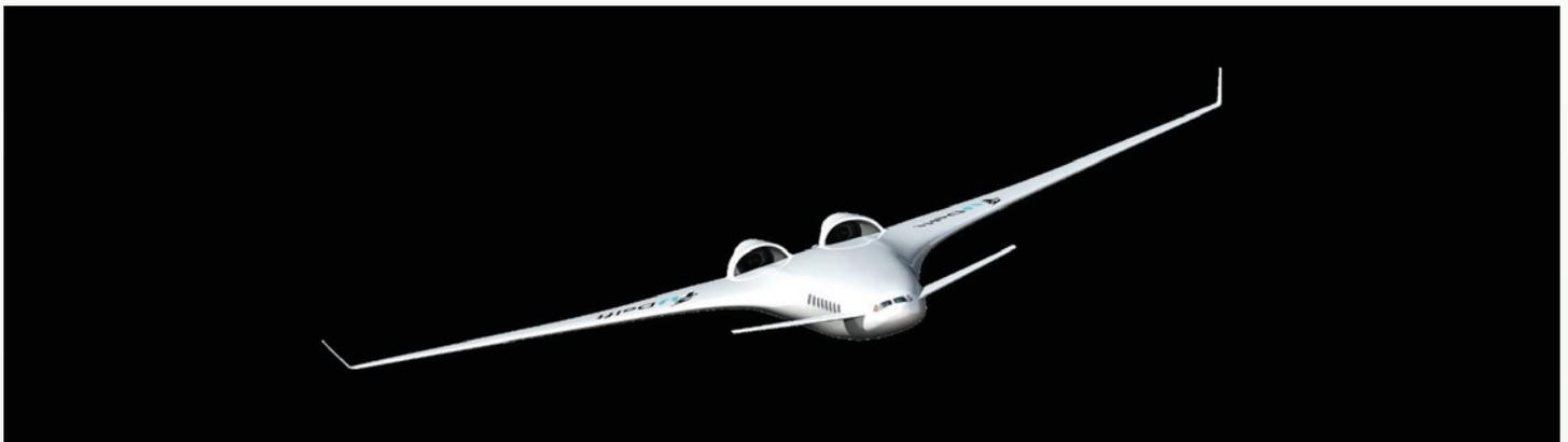
Figure 52 - Blended Wing Body (BWB) concept developed for the AHEAD project [17]
