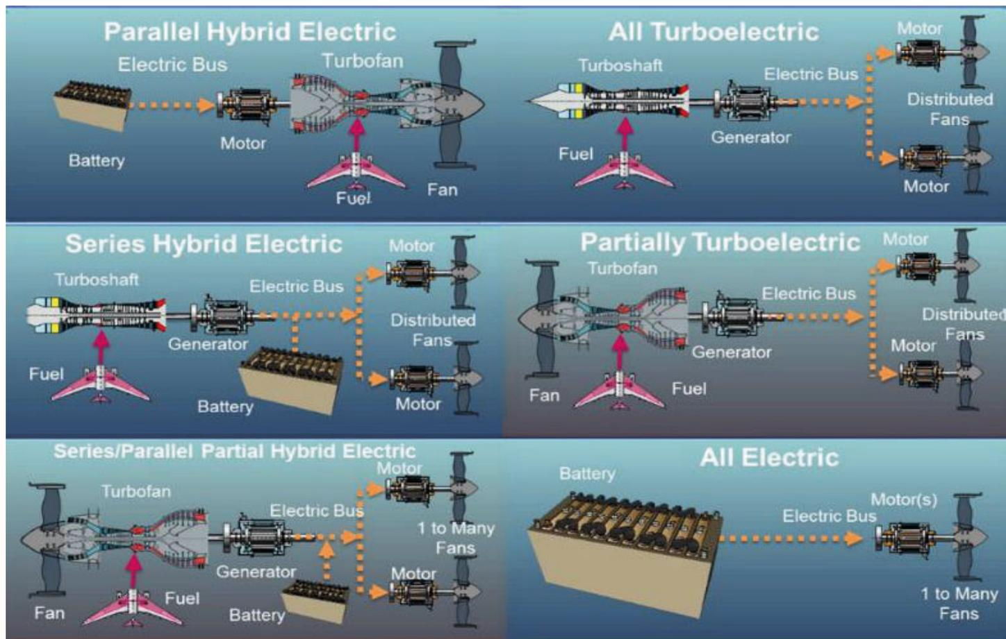
Figure 98 - Felder's classification of power system architectures for aircraft electric propulsion [15]
