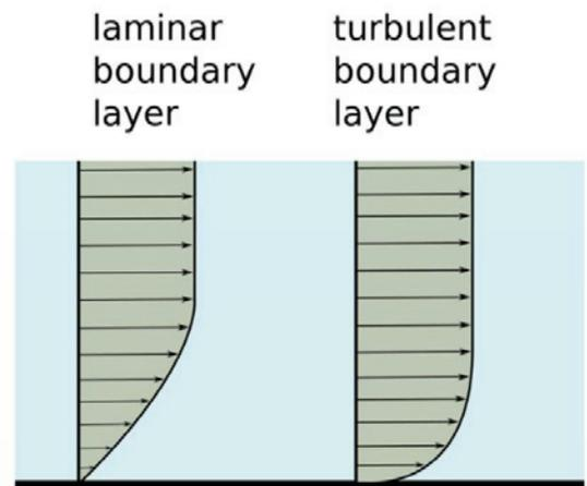
Figure 42 - Difference between laminar fluid flow and turbulent fluid flow, showing the different shapes of the developed boundary layer [10]
