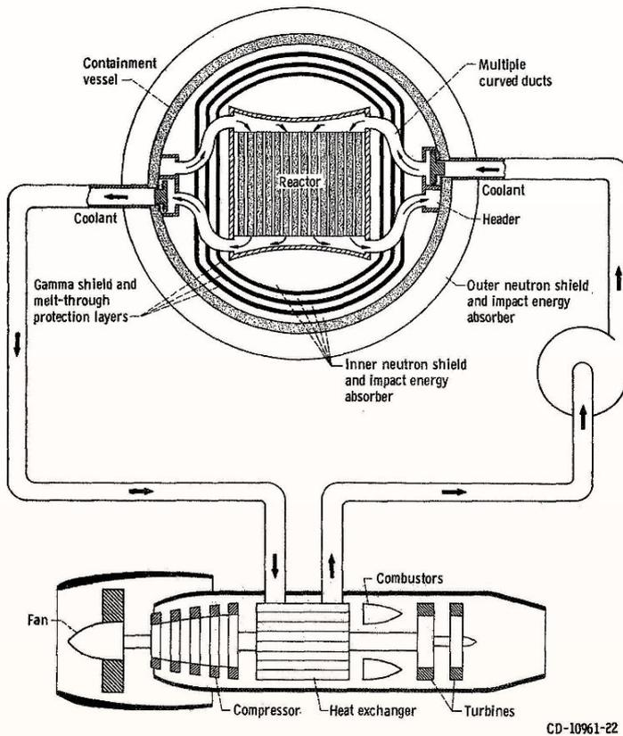
The principle of a fission reactor consists of a core containing nuclear fuel, uranium. The reaction of fission produces heat. This heat is absorbed by a coolant. Depending on the option, either the coolant can exchange heat in the aircraft jet engine to produce thrust (Figure 150), or, the coolant can be refreshed in a turbine to produce the electricity used in the electric motors [02].
