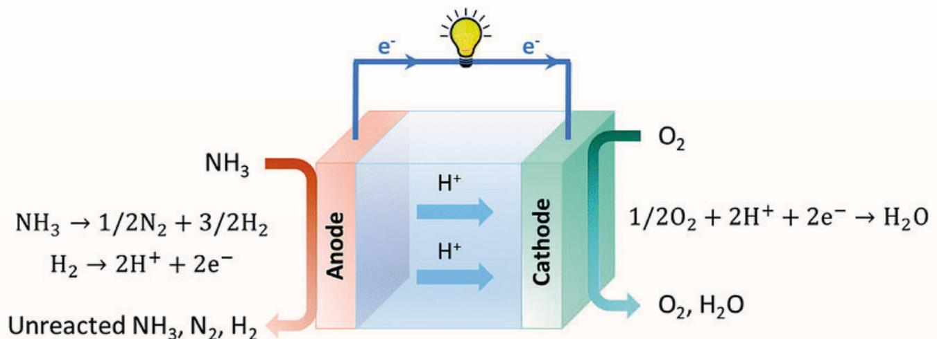
Figure 139 - Simplified view of SOFC-H
