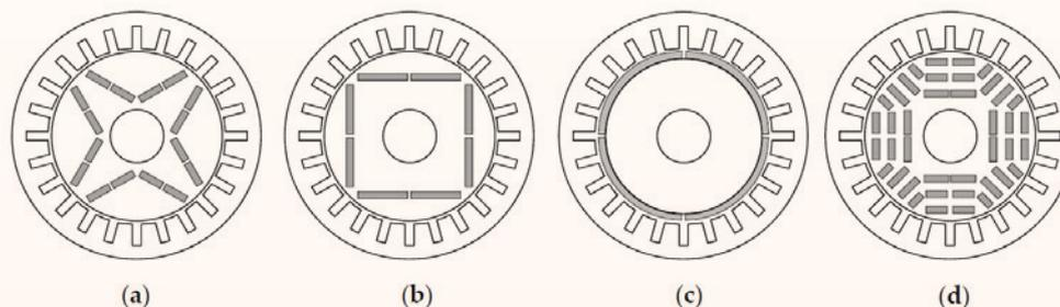
Figure 85 - Different rotor concepts of permanent magnet synchronous machines [18]:
