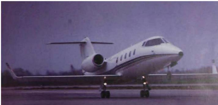
Figure 66 - Learjet Longhorn 50 series equipped with winglets [06]
