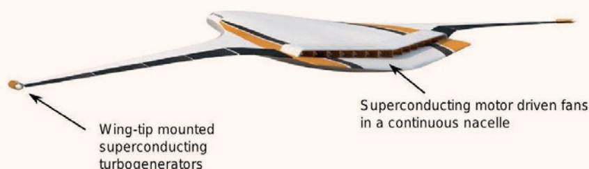
Figure 103 - NASA CONCEPT: N3-X Distributed Turboelectric Propulsion System. (Credit: NASA)
