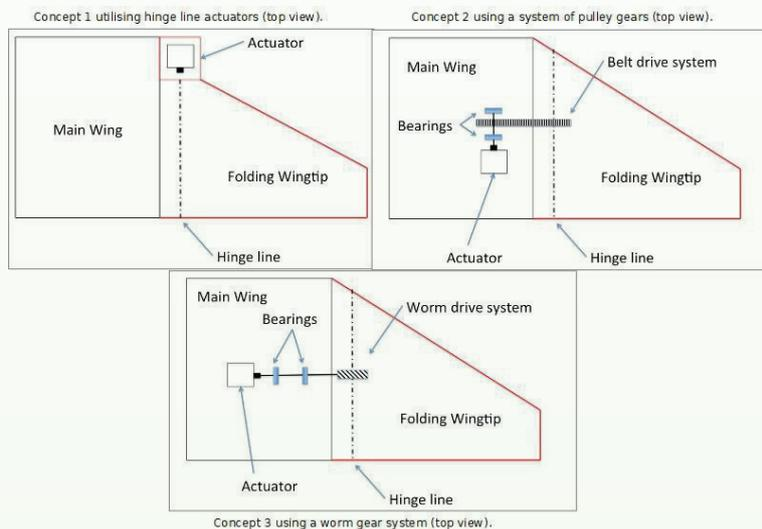
Figure 73 - FOLDERONS Hinge actuator concepts [14]
