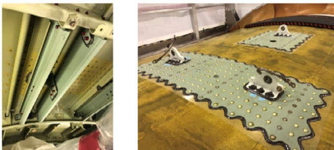
Figure 3 - Renforts structure – internes (intercostal) / externes (doubleurs)
